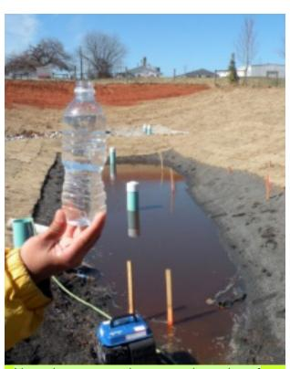
Note the contrast between the color of the runoff in the pond before it has been filtered and the clear water in the bottle, after it has been filtered through the Stalite fines
